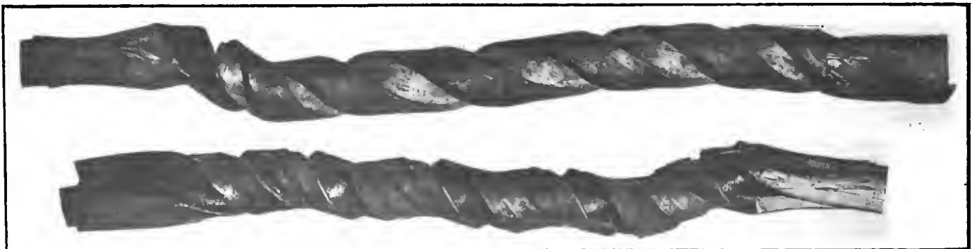
Fig. 2.—Specimens of automobile front axles after the torsion test has been applied
